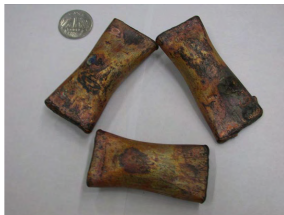
Fig. 4. Photograph of copper jacketed as cast U–Mo alloy samples.
